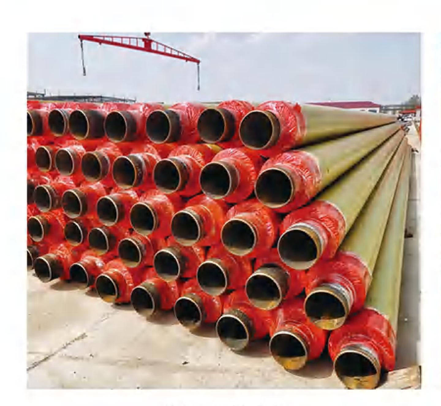
黄夹克保温钢管 Yellow jacket thermal insulation steel pipe
