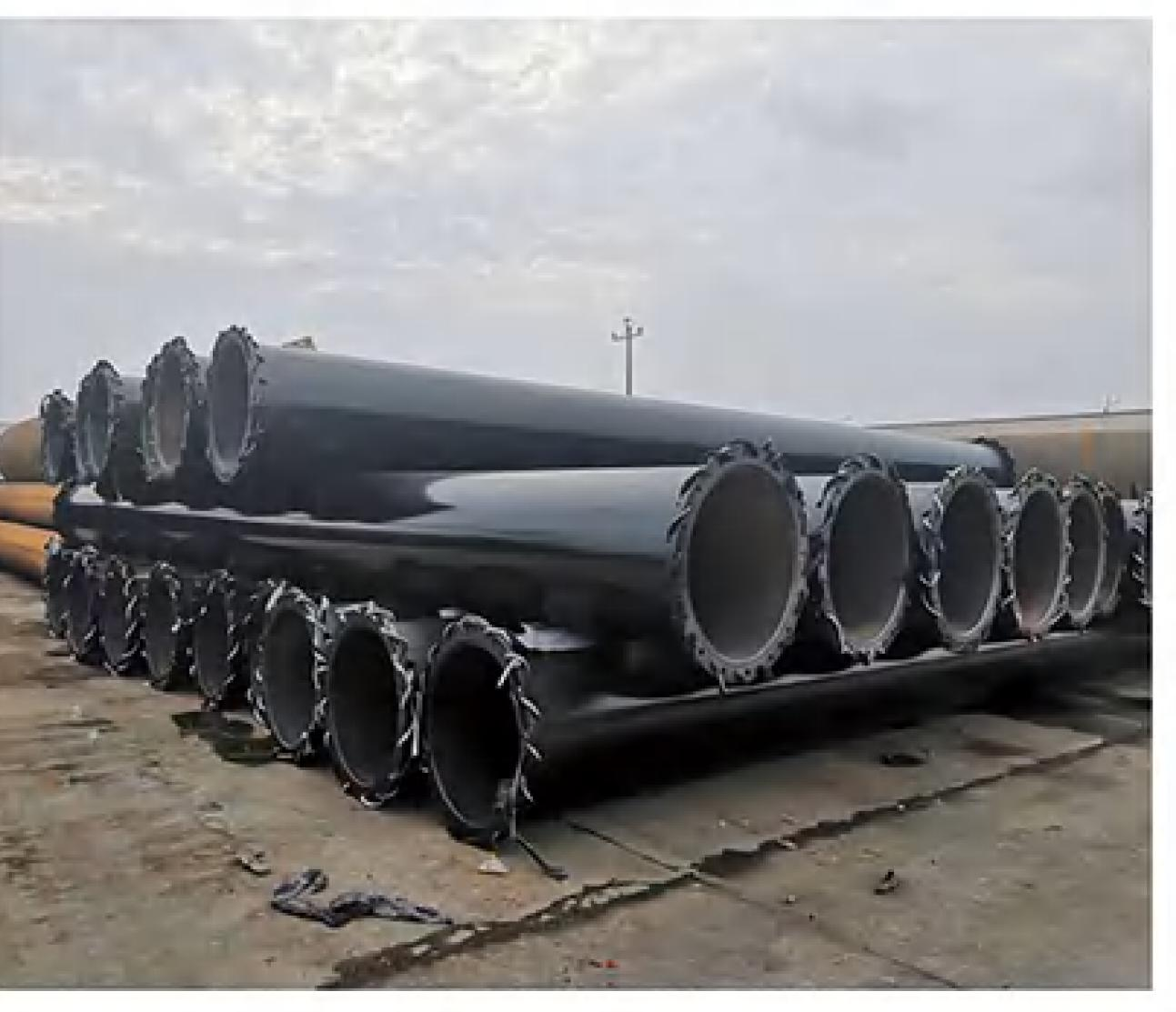
FBE 防腐 FBE anti-corrosion
