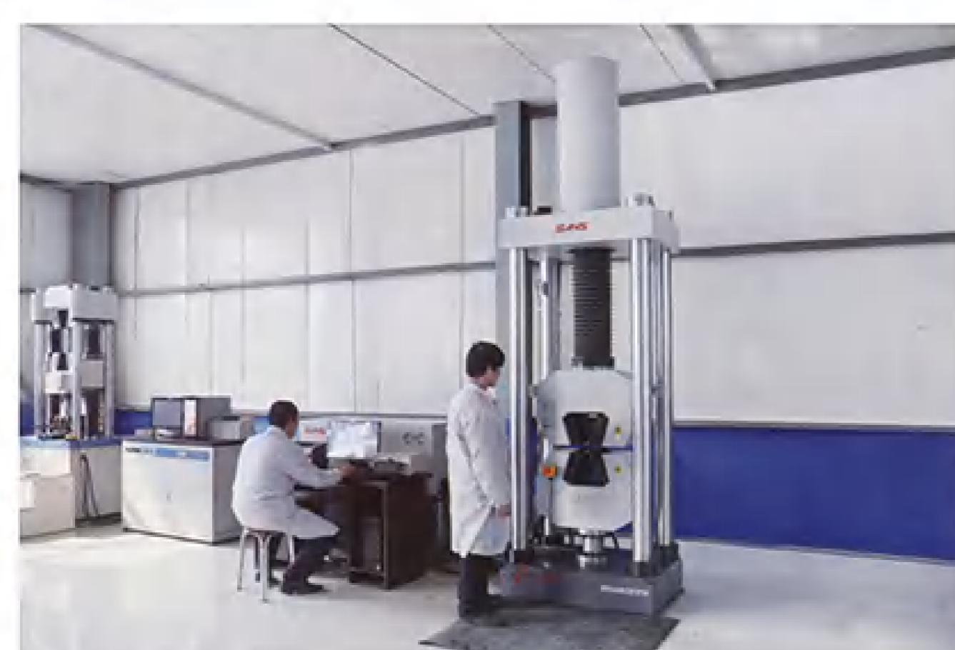
1000KN微机控电液伺服万能试验机 1000KN Electro-hydraulic Servo Universal Testing Machine
