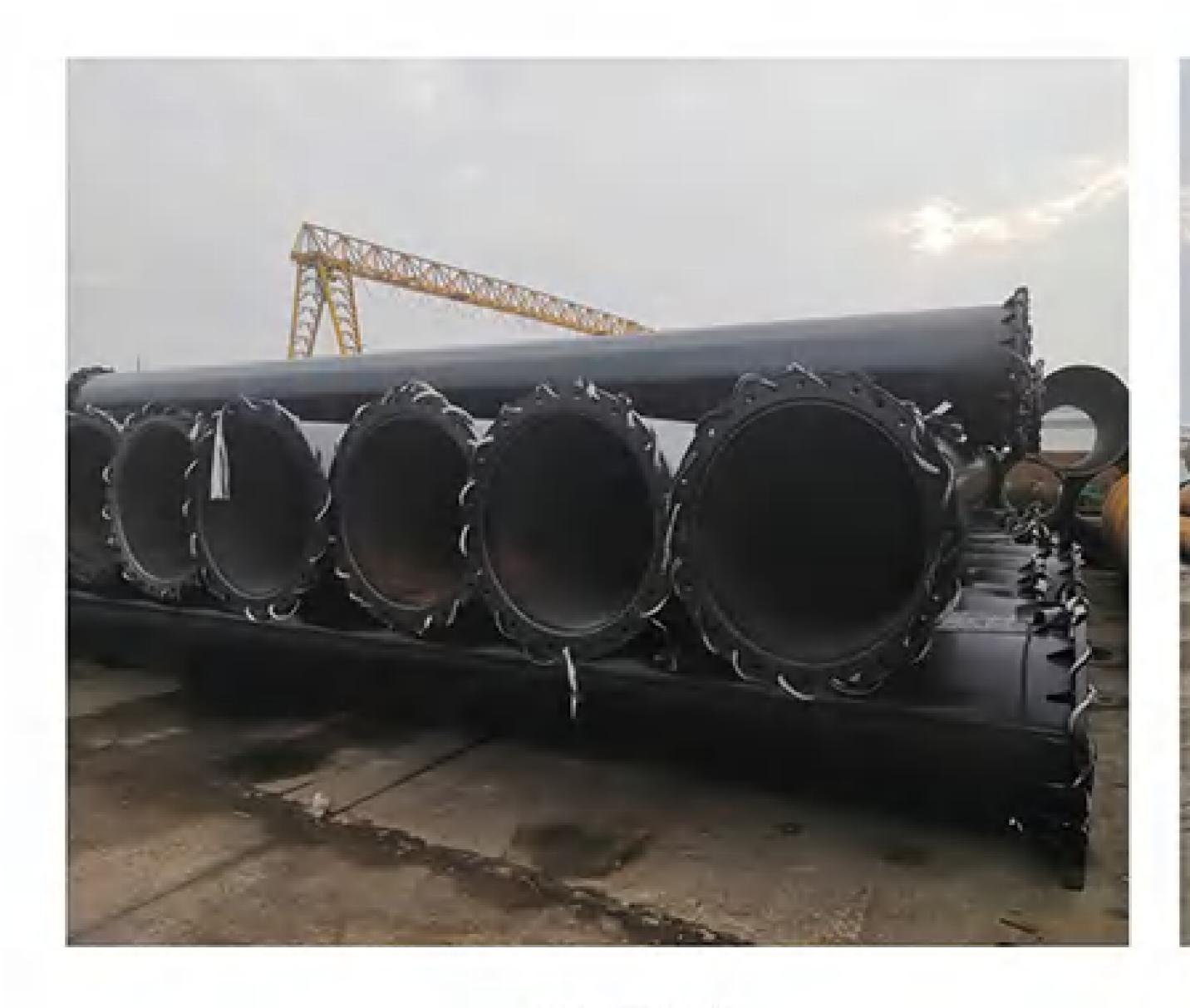
FBE 防腐 FBE anti-corrosion
