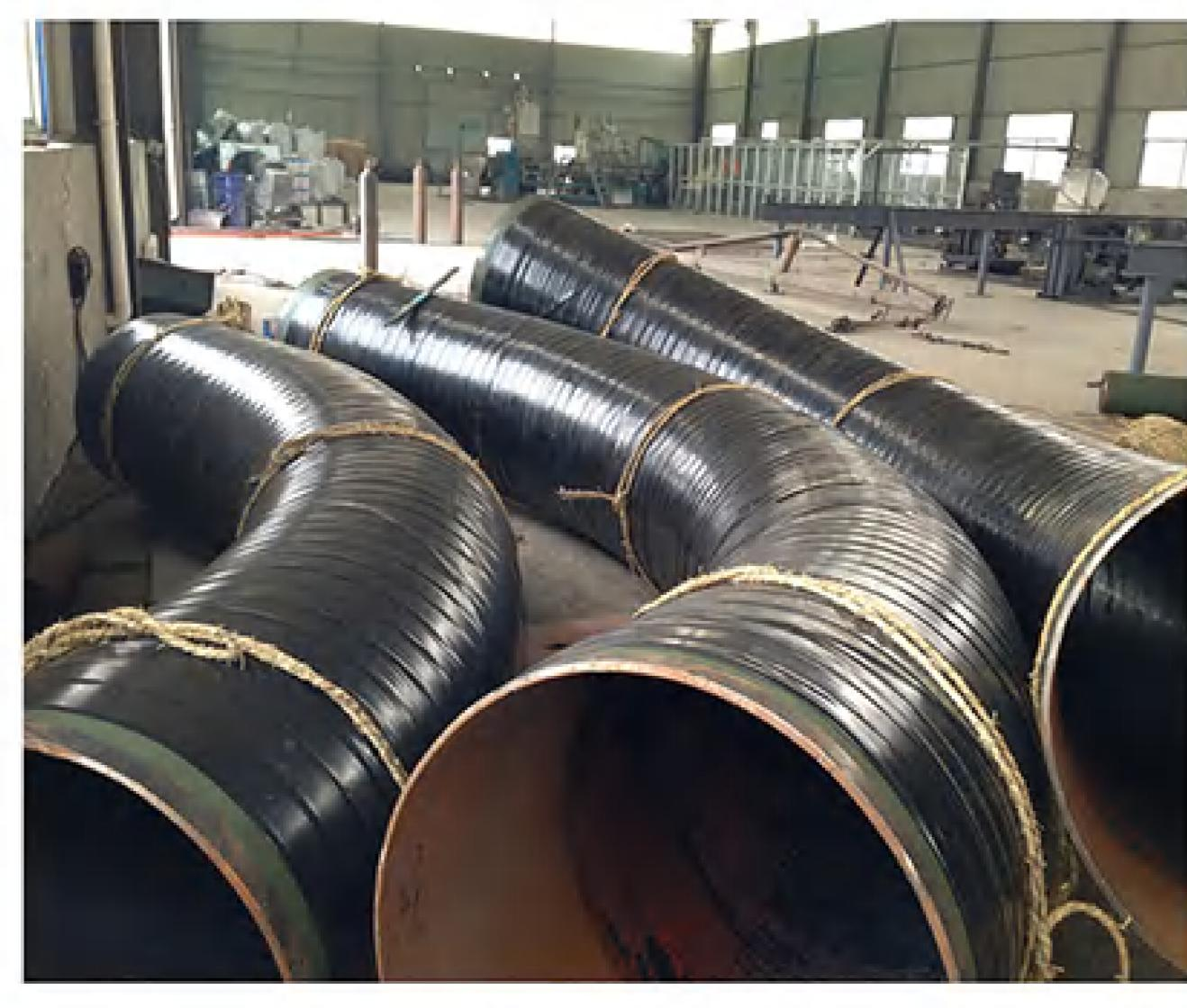
手缠热缩带防腐弯管 Hand Wrapped Heat Shrinkable Belt Anticorrosion Bend
