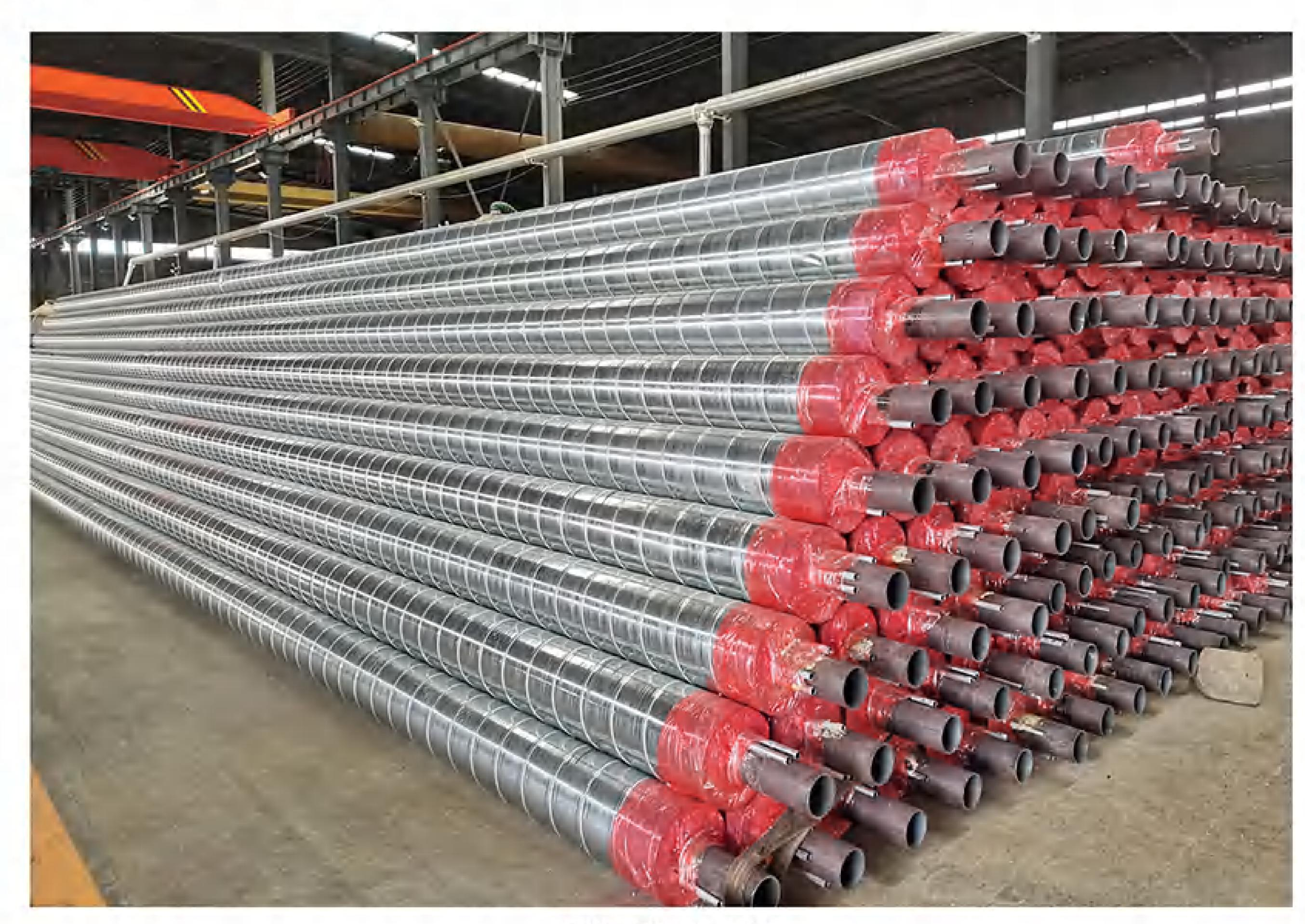
镀锌铁皮保温钢管 Galvanized iron sheet insulated steel pipe
